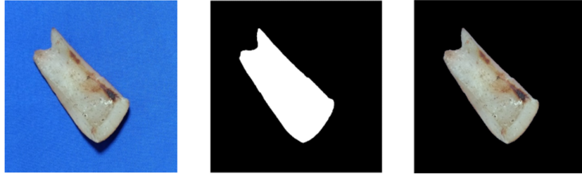
Figure 2.1: Background removal by segmenting the background and the copra using thresholding [1].
